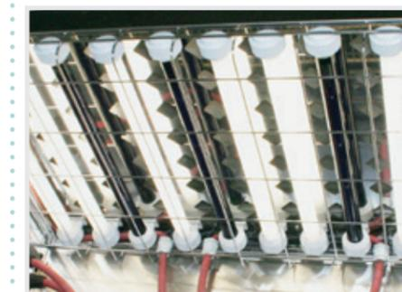
Chamber with combined or separated VIS-UV source of light with independent control and automatic assessment of photo stability test.
