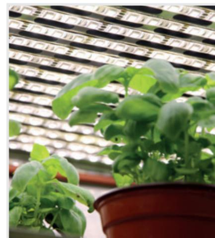
Exact growth chamber with variable growth height and full-spectrum fluently controllable LED lighting.
